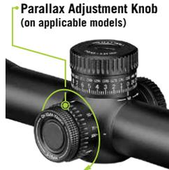
Dial the Parallax Adjustment Knob until the target image is as sharp as possible. The yardage numbers on the knob should be used as general reference points only. Check for parallax error by moving your head up, down, left, and right without influencing the gun. The parallax is correct if there is no apparent shift between the reticle and the target image. If you notice any shift, adjust the focus knob slightly until all shift is eliminated.
