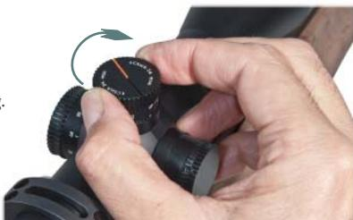
Turn the elevation knob a partial turn in a counter-clockwise direction until the Radius Bar is correctly aligned with scope axis and zero marks match. This setting will match the original zero point.
