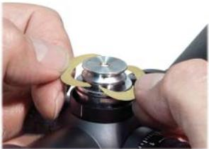
Use as many shims as necessary to completely fill up the space. Do not try to force in a last shim once the clearance is very close.
