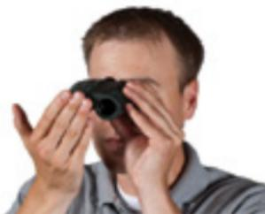
**Adjust the diopter:** Start by closing your left eye or covering the left objective lens with your hand. Lift the diopter ring to unlock and, looking through your right eye, adjust the diopter so that the object is in focus. Make note of this diopter setting in case you need to set it again. Push the diopter ring down to lock—from this point on, you will only need to use the center focus wheel.
