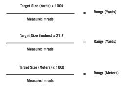
Using either the vertical or horizontal mrad scale, place the reticle on the target of known dimension and read the number of mrads spanned. Obtain maximum accuracy in ranging by calculating exact mrad measurements—try to estimate mrad measurement in 1/10s if possible.
