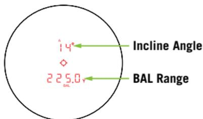
The slope incline number can be entered into ballistic programs or field cards to help calculate precise bullet drop in mountainous terrain. This number is automatically calculated into the wind/drop solution provided in the display and in the app. See Ballistics Manual for more information about the ballistic information displayed.
