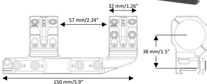
The **IDEAL SCOPE MOUNT SYSTEM** series of mounts feature **seven set of interfaces** to **attach any of more than 40 different accessories** and has a bubble level integrated in the rear plane of the mount body to prevent canting of the rifle. The rings are diagonally cut for increased visibility of the elevation and windage turrets (US Patent 8,733,011).
