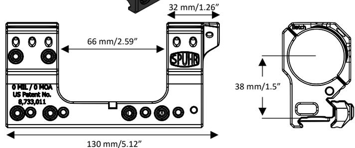
The **IDEAL SCOPE MOUNT SYSTEM** series of mounts feature **seven set of interfaces to attach any of more than 40 different accessories** and has a bubble level integrated in the rear plane of the mount body to prevent canting of the rifle. The rings are diagonally cut for increased visibility of the elevation and windage turrets (US Patent 8,733,011).
