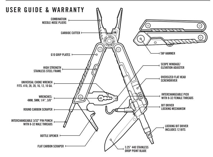
**PLIERS:** The combination needle-nose pliers are made to get a grip during any situation. Their highly functional shape allows for fine work with the tip as well as bigger, more aggressive tasks towards the back of the jaws. The carbide cutter is designed to cut most common gauges of copper wire.
