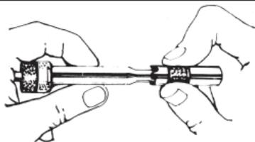
Lock deprimed case in shell holder with the lock stud. Insert pilot into case with pin in flash hole and rotate until it stops cutting. If no metal is removed, case does not need trimming.
