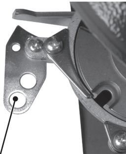
**ACTION ROD INSTALLED HERE**
