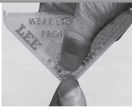
Slide the flow control to **LOCK** position, feel for the detent. Grasp the top and bottom of the flow control valve using your thumb and index finger above and below tray. **NOTE:** Make sure it is in the **LOCK** detent position, else primers may spill.
