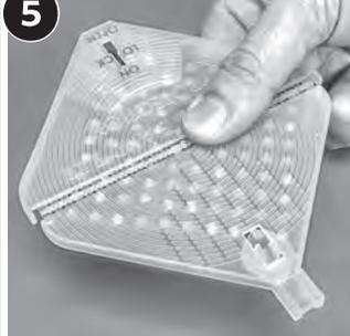
Unfold tray and place on top of box of 100 primers.
