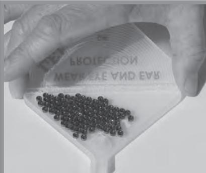
**6** Lift tray so output spout touches table, shake tray side to side to upright all the primers. Allow cover to naturally fold up, notice how the primers glide across hinge, upright themselves and work their way towards the outlet. Fold and close cover.
