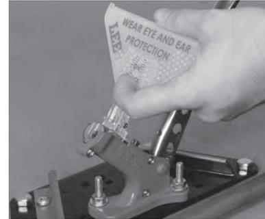
**7** Slide the primer tray into the adapter, slide the flow control to **ON**, and watch the flow of primers from tray into adapter. Primers may bridge, tap the upper corner of tray occasionally to resume flow.
