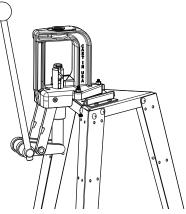
Step 6: Slide your press into the Z-brackets and tighten the four Z-bracket screws. To remove press, loosen Z-bracket screws a turn, and slide from the brackets.
