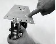
Step 3: Insert qty. 3, 2" long, 1/4"-20 elevator bolts (sold at any hardware store or McMaster-Carr®). into wood block, and tighten bolts until flush with wood block.
