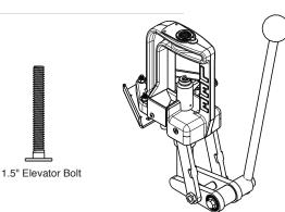
Step 5: Secure Lee press to steel base block using three 1.5" elevator bolts, 1/4"-20 washers and 1/4"-20 nuts. If you need to mount another manufacturer's press, see instructions (RIGHT) on mounting to your own wood block.
