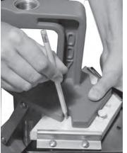
Step 2: Use press frame as drill template, and mark holes. Loosen Z-bracket screws, and remove wood block. Drill mounting holes.
