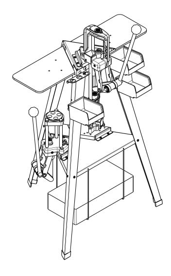
4" x 8" x 16" concrete min. block not included, but necessary for safe, stable operation. Stand is sized to accept up to 10" x 8" x 16" block. Obtain one at any building supply or home center.
