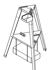
Step 4: Attach concrete block hangers to intermediate plate as shown. Install concrete block. Fasten steel Z-Brackets to top-plate using provided 1/4"-20 Phillips Pan HD. Attach bin bracket and bin on desired leg, using the provided 1/4"-20 Phillips Pan HD and 1/4"-20 nuts.
