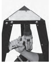
Step 1: Secure wood block into Z-brackets on the top plate. Using a <sup>1</sup>/<sub>4</sub>" or larger drill bit, drill both alignment/ lock holes.
