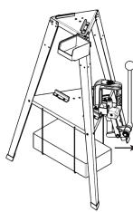
To remove press. grab press below level of intermediate plate and pull straight out. The intermediate plate is intended only for press storage, it is not designed to be used as a platform for reloading operations.
