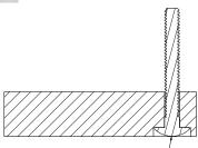
HEAD OF FASTENER CANNOT PROTRUDE PAS BOTTOM OF WOOD BLOCK
