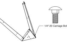
Step 2: Place two legs down on a level surface and attach legs to top plate using supplied 1/4"-20 carriage bolts and 1/4"-20 nuts. Finger tighten 1/4"-20 nuts on carriage bolts.
