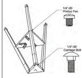
Step 3: Attach intermediate plate to leas using provided 1/4"-20 Phillips Pan HD and 1/4"-20 nuts. Install third leg using remaining 1/4"-20 carriage bolts.
