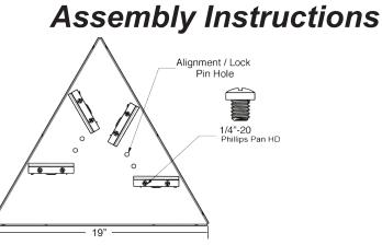
**Step 1:** Fasten steel Z-brackets to intermediate plate using provided 1/4"-20 Phillips Pan HD.
