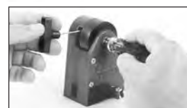
Polish case with steel wool, scouring pad or crocus cloth
