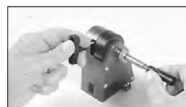
Trim the case using the Lee Case Trimmer
