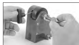
Chamfer the case inside and out
