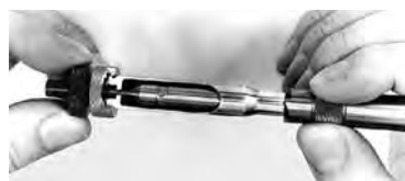
Lee Case Trimmer Simplest and safest way to check the case and trim to the correct length.
