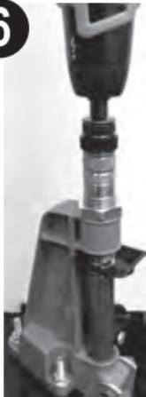
4) Install Quick Trim die into press according to instructions included with die. Raise ram to insert case into die.
