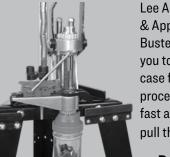
Lee App press & App Bulge Buster kit allow vou to automate case feeding and process cases as fast as you can pull the lever.
