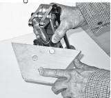
Make sure the wood block is right side up, so that the alignment holes in the wood block and the steel plate line up. Select the appropriate length elevator bolts and secure press to base block. Tighten nut until the flat head of the bolt is flush with wood base.
