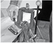
Slide your press into the Bench Plate. Insert a 1/4" bolt, screwdriver shank into the lock/alignment hole. This ensures the wood block is properly aligned and will not slide out during your reloading session. Tighten the four Z-bracket screws. To remove press, loosen Z-bracket screws a turn, remove lock/alignment pin and slide from the base plate.
