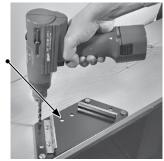
Install the Z-brackets with the provided 1/4"-20 pan head screws. Start the screws in a few threads, but do not fully tighten at this point.
