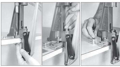
ATTACH your press with (3) 1/4" bolts. Use 'T' nut for quick removal to empty spent primers. NOTE You may drill a hole through the bench and catch the primers in a container below.
