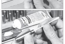
Be sure to lube the inside of the case neck with a cotton swab. Lee Resizing Lubrciant # 90006
