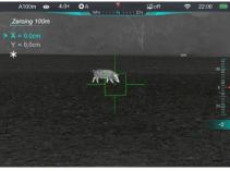
the **Controller (4) + Power button (5)** at the same time until a snowlike freezing icon **\*** appears on the left of the screen, and the image is frozen.
