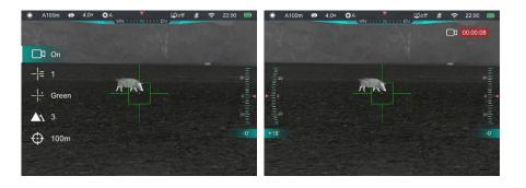
• The recording icon and prompt box showing the recording time appear in the upper right corner of the display, with the time format as 00:00:00 (hour: minute: second).
