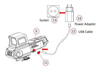
**Note:** 1. When the USB-C cable is used for power supply, the USB-C cable will be preferred for power supply, and the battery will be stopped. 2. The product supports 3V and 3.7V batteries. To ensure the correct display of the power level, please select the correct battery voltage in the menu.
