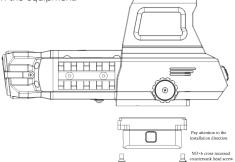
• Fixing Fast requires the use of recoil-absorbing mount provided in the packaging, as follows:
