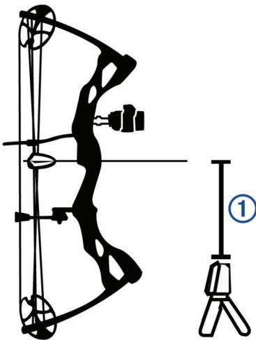
The device detects shots and displays measurements automatically as you shoot. The measured velocity is the speed of the arrow as it passes over the chronograph.
