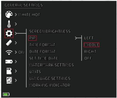
The user has the option to place the PIP window in the upper left/middle/right area of the display.
