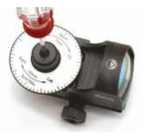
One scale division of this disc (or tick mark) corresponds to 1 minute of angle (MOA), or approximately 1 inch at 100 yards. For other distances, this value is proportional, for example: .5 inch at 50 yards or 0.1 inch at 10 yards. Before shooting, make sure to tighten the lock screws on the rear of the FastFire 2 with the provided screwdriver, making sure not to over-tighten.
