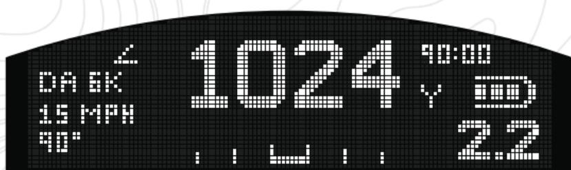
The XTR PS features a built-in, heads-up display that shows elevation turret position in yards, meters, or MIL; rifle cant (bubble level); user-defined wind speed; user-defined wind direction; distance-accurate wind holds; a user-selected density altitude table; a battery meter; and a match timer.
